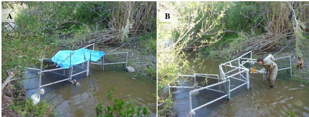
Figure 2- 6. Downstream and Upstream migrant weir traps at 1.3 RKM (A) with and (B) without cover (used from fall 2010-present).
