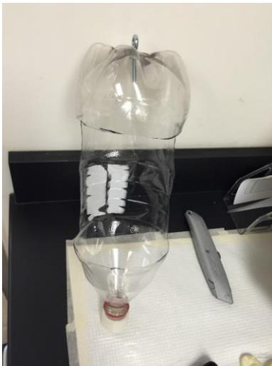
**STEP 4.** Insert eye bolt and secure nut to hole. Put 1 cup of water and 5 drops of Dawn dish soap into the 16 oz bottle. Twist on either a 3D printed connector (available upon request from the RCDSMM) or use a small 2 inch wide radiator screw clamp to connect the opening of the 2L bottle with the opening of the 16 oz bottle.
